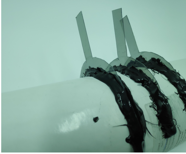
(a) Closeup of polarizers inside the cardboard cylinder.
